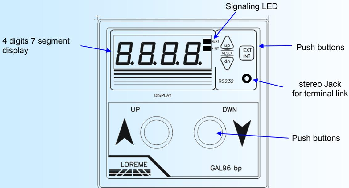
The front face of the device is composed of:
